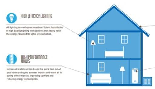
These are cost effective measures that home builders may consider to achieve new levels of efficiency. They can be traded for other efficient technologies such as higher efficiency HVAC units, higher efficiency water heaters, etc.
