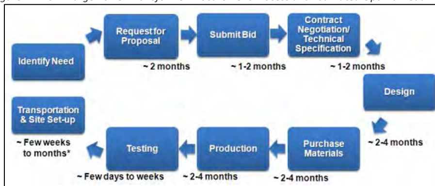
Figure 17: 2011 Large Power Transformer Procurement Process and Estimated Optimal Lead Time
