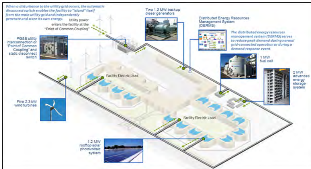
Figure 26: Commercial Microgrid Application at Santa Rita Jail in California
